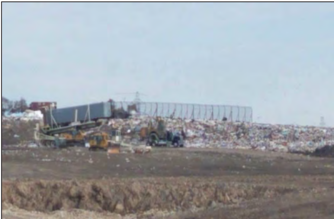
Tipper in center of waste placement
